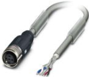
Bus system cable, CANopen®, 5-position, PUR halogen-free, Gray RAL 7001, Free cable end, on Socket straight M12-SPEEDCON, A-coded, Cable length: 2 m
